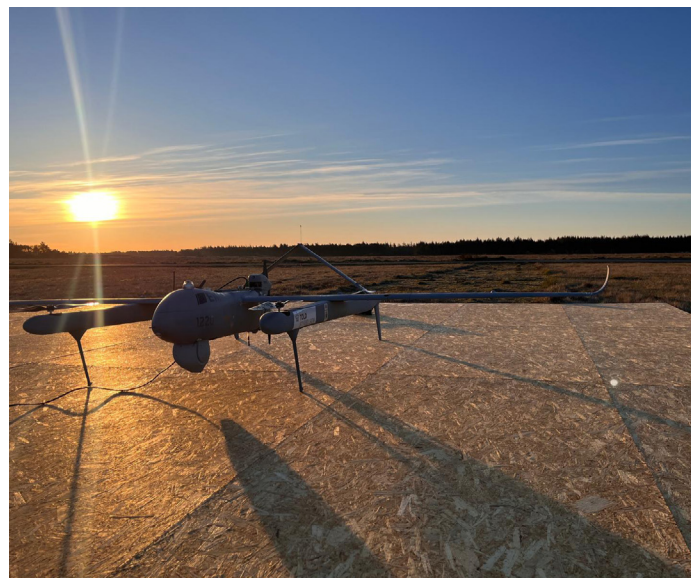
The RPAS deployed in Denmark has infrared and optical cameras and is also equipped with an embedded automatic maritime scanning sensor.
