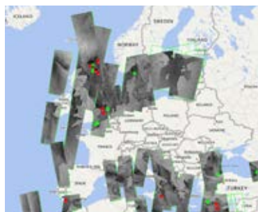
The CleanSeaNet service is based on the regular ordering of Synthetic Aperture Radar satellite images, providing coverage both day and night, and independent of fog or cloud cover.
