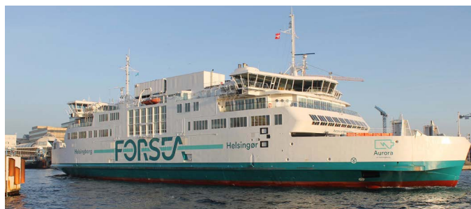
The ferry Aurora of Helsingborg at the port of Helsingborg. The ferry is one of the first in the world that is powered by battery.
