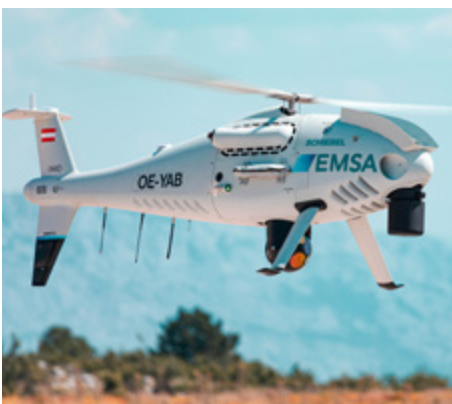
The EMSA RPAS services have been developed to assist in maritime surveillance operations to support authorities involved in Coast Guard functions undertaken by Member States
