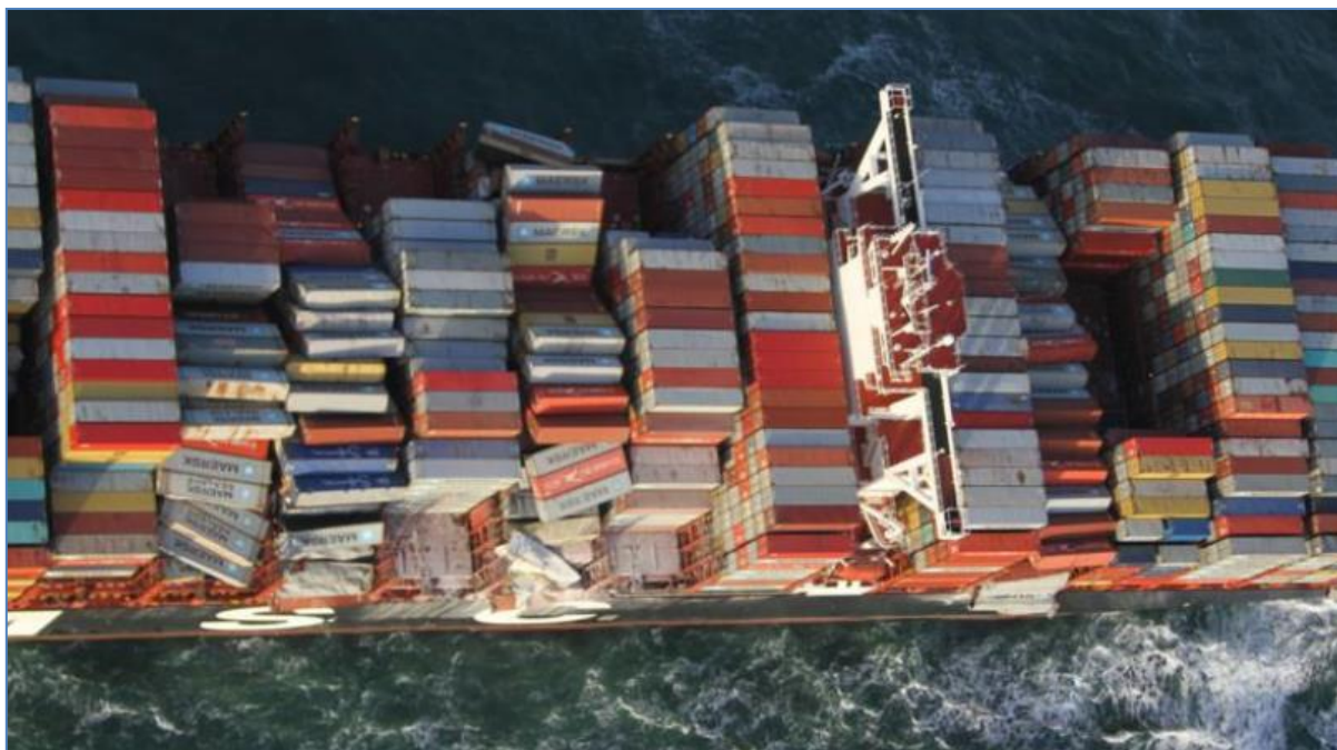
Figure 1 - Top view MSC Zoe following the loss overboard of containers (Source: BSU / Netherlands Coastguard)
