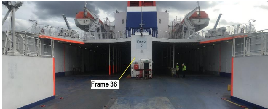
Figure 31: Picture of the aft openings on the Ferry RoPax ship.
