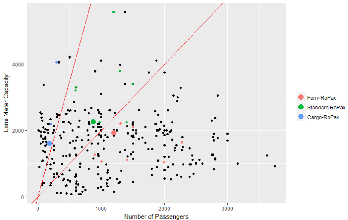
Figure 4: Lane meter capacity vs. number of passengers for the FIRESAFE II fleet (in black) and the Stena fleet (in colour) and FIRESAFE II groups (red lines)
