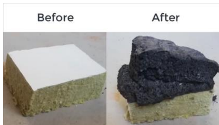
Figure 121: Intumescent paint before and after heating.
