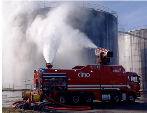
Figure 115: Water mist turbine performance test.
