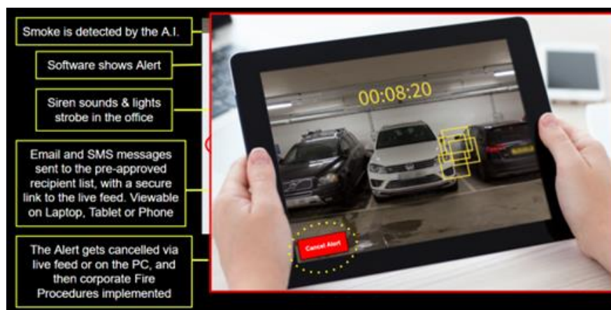
Figure 99: AI based smoke detection system and its user interface
