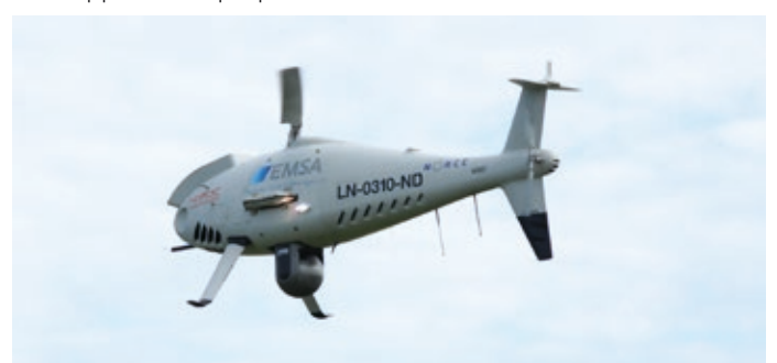
EMSA RPAS are equipped with special gas sensors which can measure the amount of SO x and NO x emitted in the plume of a ship and in doing so indicate possible cases of non-compliance for follow-up by port authorities
