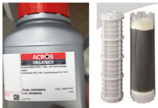
Figure 11 - Ion exchange resin (left), cartridge nylon (middle) and activated charcoal cartridge (right)
