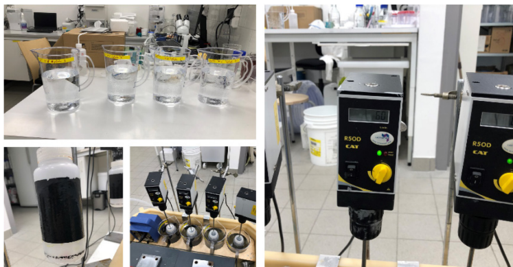
Figure 15. From left to right, from up do down: The release rate measuring tanks; the rotating device for biocide extraction at 60 rpm; the cylinder painted on a 200cm 2 area and the extraction moment in the water bath at 25^{\circ}\text{C} \pm 1^{\circ}\text{C} .
