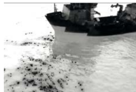
Oil detected by an RPAS infrared camera
