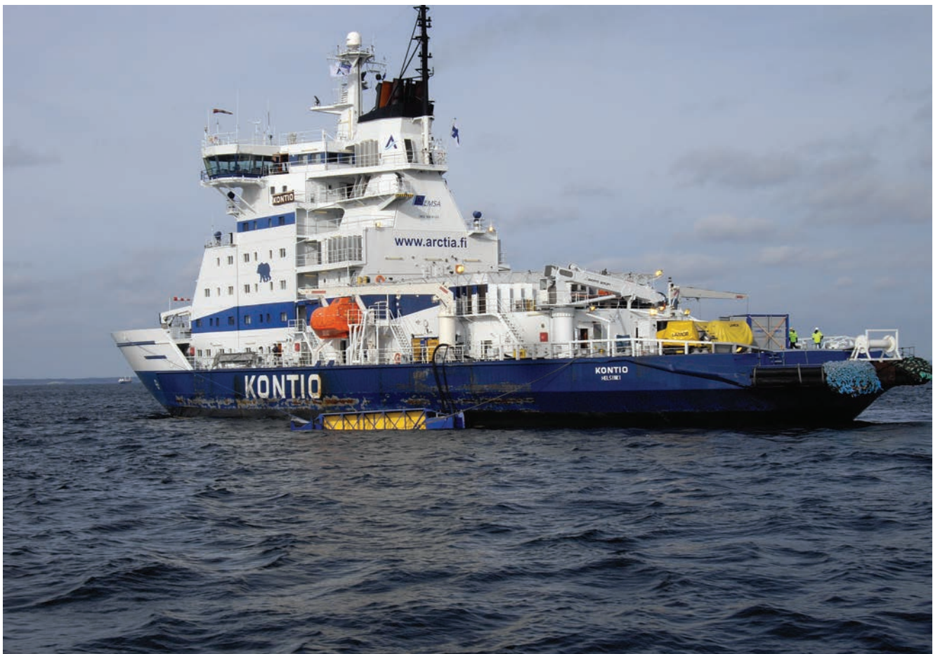
EMSA contracted ice breaker Kontio with deployed sweeping arm during the CEX-11 exercise.
