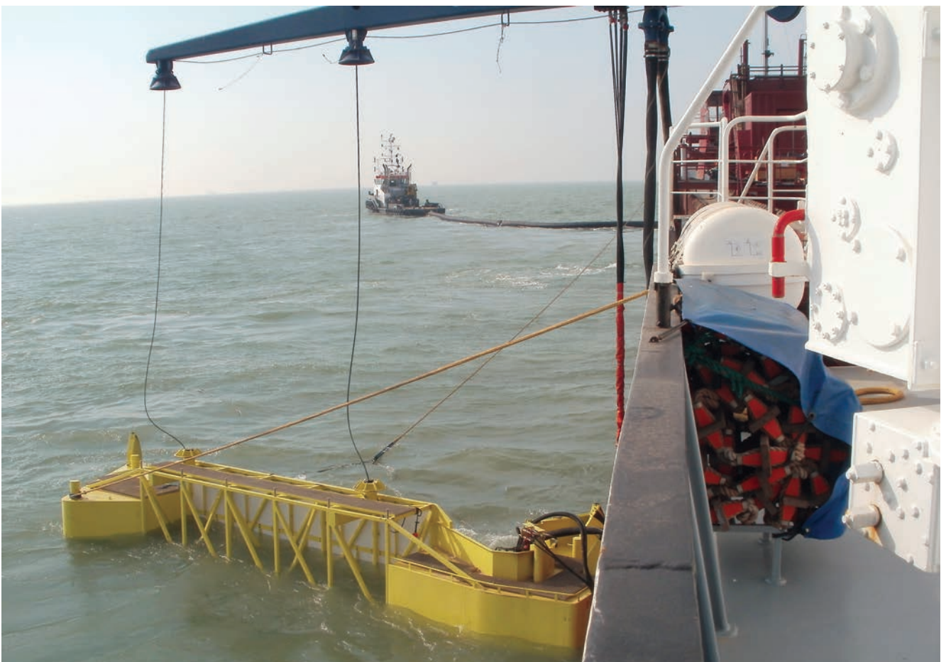
DC Vlaanderen with port sweeping arm following the oil collection boom during the joint exercise with The Netherlands and Belgium.
