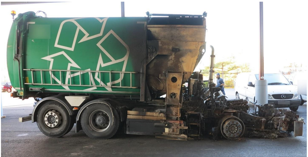
Figure 6: Garbage vehicle where the cab and front tires have been completely consumed in a fire, but the rear part of the vehicle was not involved as it is primarily made from steel. Photo: RISE.
