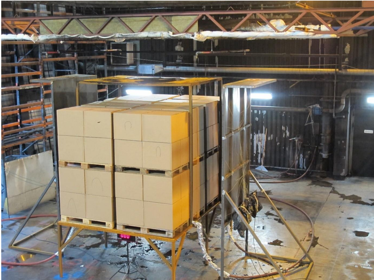
Figure A2-1: An illustration of the arrangement of the commodity on the trailer mock-up, the roof over the central 2 by 2 stacks of commodity and the steel screens alongside the set-up.
