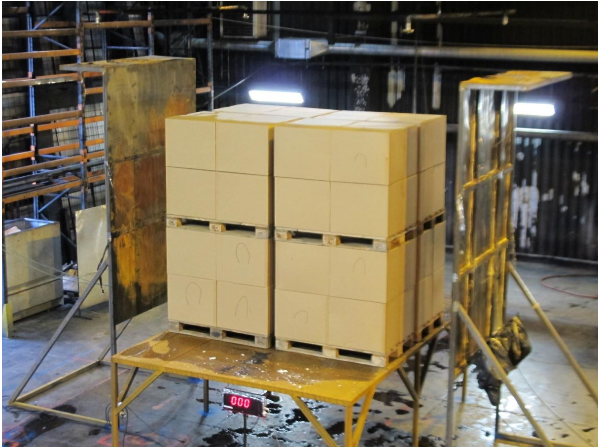
Figure A2-3: The altered test set-up used in Test 5, where the roof over the central 2 by 2 stacks of commodity was removed and the outmost stacks of commodity not were used.
