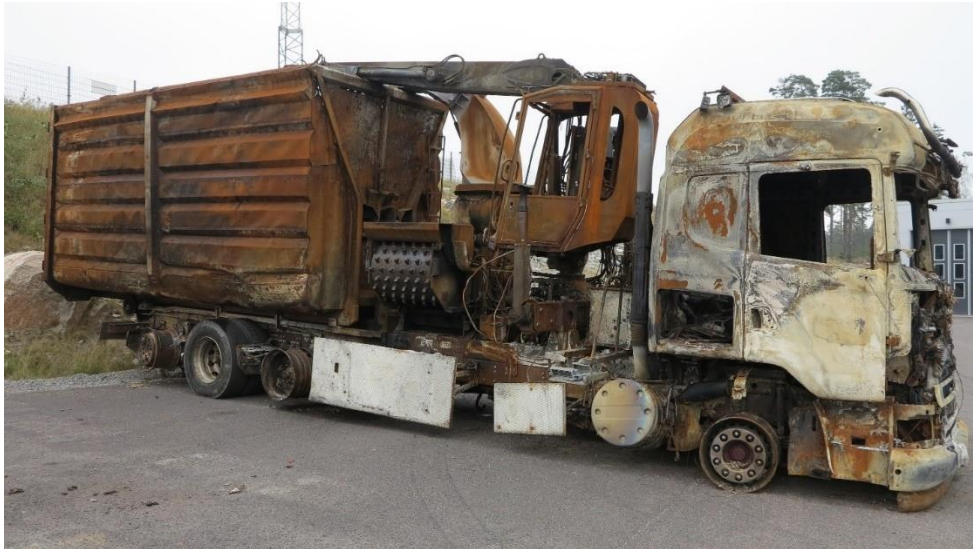
Figure 7: The results of a fire in a wood chipper vehicle. It is likely that the fire started when hydraulic oil leaked and ignited on a hot surface. It can be observed that virtually all combustible materials have been consumed but the structure is relatively intact. The rear tires were installed after the fire to facilitate transport from the site where the fire occurred. Photo: RISE.
