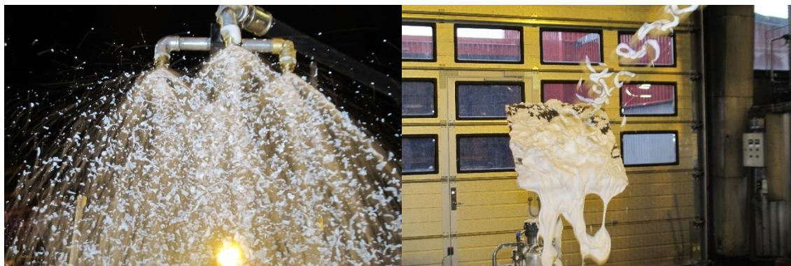
Figure 9: A multi-orifice CAFS nozzle under operation and the foam quality from a hand-held nozzle demonstrating a certain adhesion to vertical surfaces. Photo: RISE.
