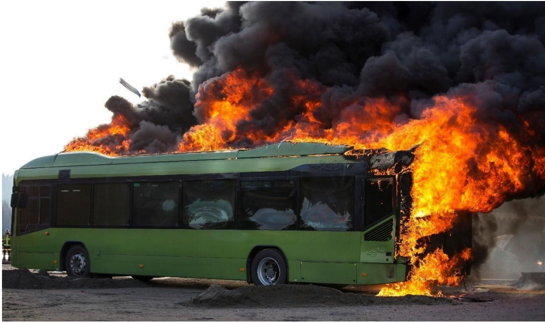
Figure 2: Fire in a bus used for city traffic. The fire was intentionally started in the engine compartment. At this stage, the engine compartment is fully involved in the fire, the interior is involved, and the center part of the roof is burnt through. Photo: RISE.
