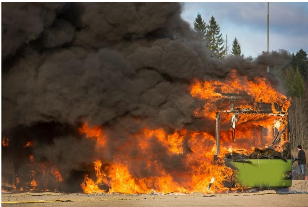
Figure 3: The fully developed fire involved the complete interior and all external combustibles including the tires. The amount of black smoke from the fire was huge. Photo: RISE.
