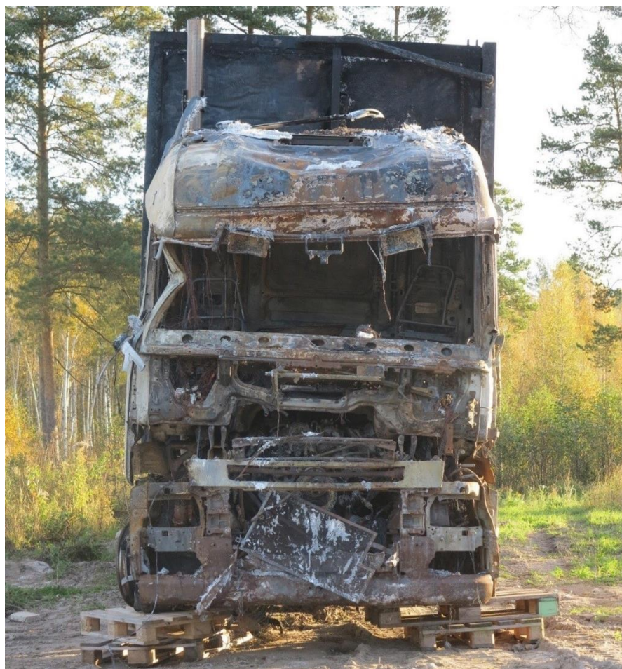
Figure 8: The result of a fire in another wood chipper vehicle that probably started in the engine compartment. It can be observed that virtually all combustible materials have been consumed but the cab is relatively intact. Photo: RISE.
