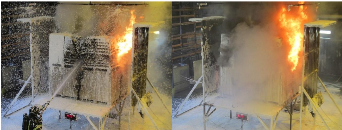
Two minutes after system activation, manual extinguishment has been initiated.
