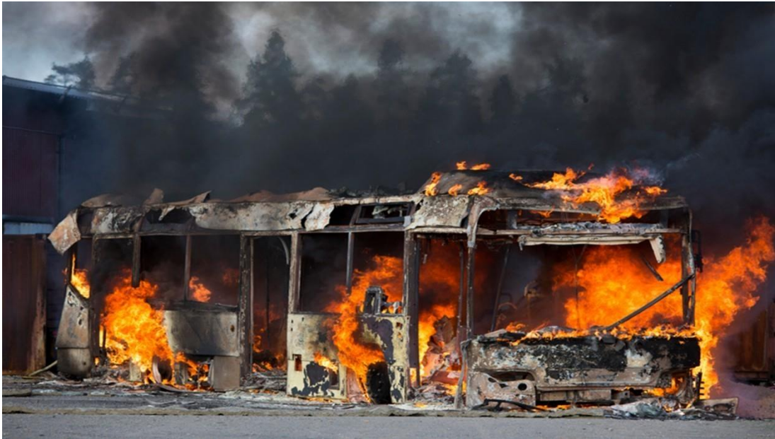
Figure 4: The remains after the test, which illustrates that all tires and the interior has been consumed. All windows and doors have broken. The body of the bus is reasonably intact, but the center part of the roof burnt through. Photo: RISE.
