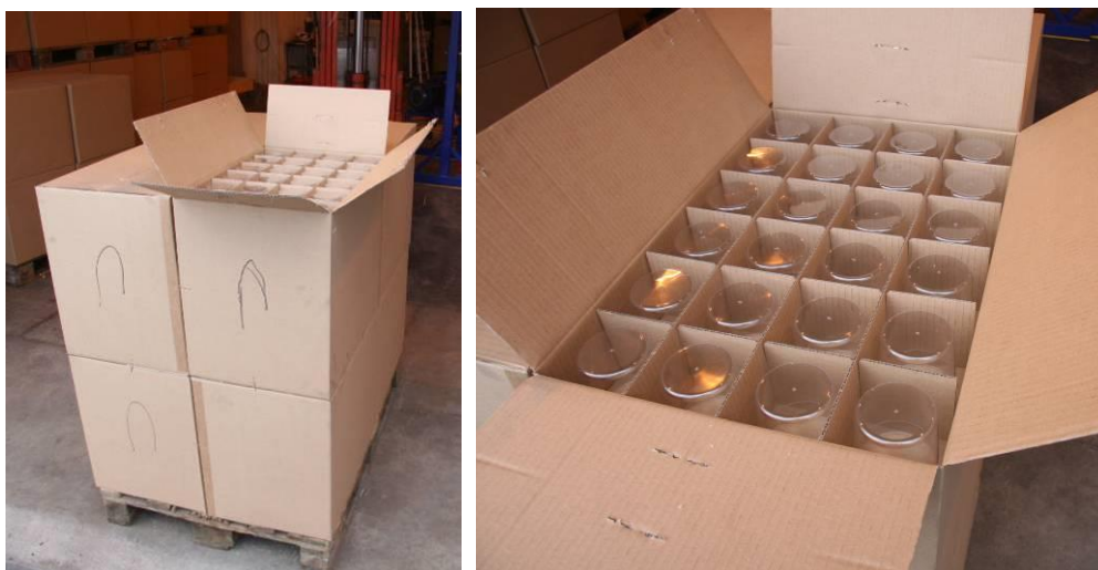
Figure A2-4: One pallet load of the EUR Std plastic commodity (left) with a close-up photo of the arrangement of the plastic cups in the individual cartons (right).
