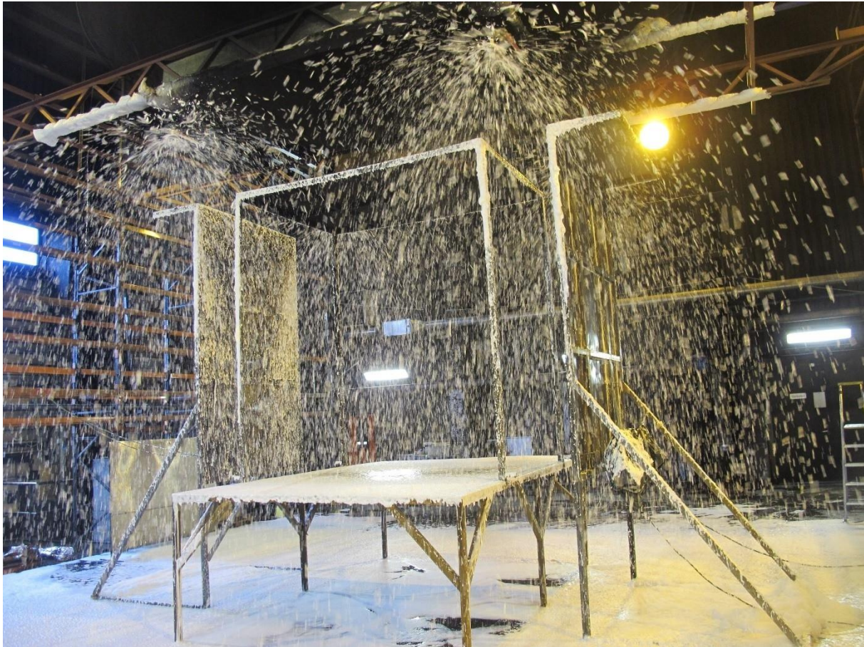
Figure A2-9: A CAF distribution test prior Test 4 confirmed a uniform distribution of foam over the test set-up.
