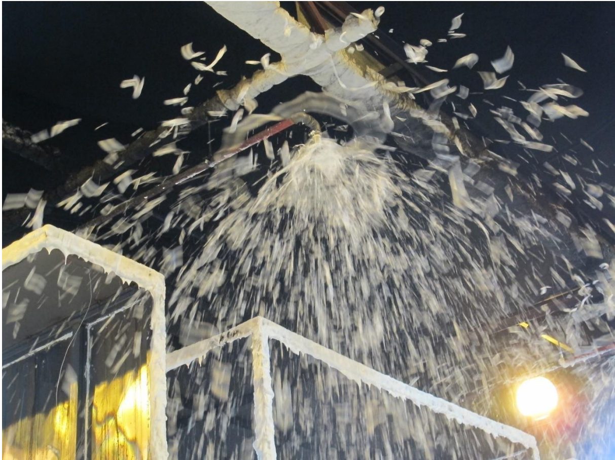
Figure A2-10: A close-up illustration of one of the rotary CAF nozzles during the distribution test prior Test 4.
