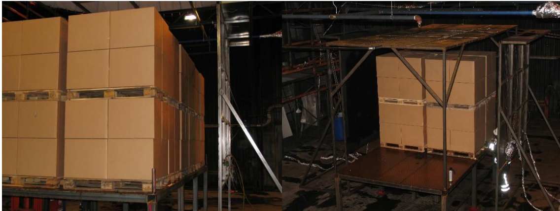
Figure 15: An illustration of the arrangement of the commodity on the trailer mock-up, showing the steel sheet screen on the right-hand long side. A similar screen was positioned on the left-hand side. The photo to the right shows the trailer mock-up with the roof installed. Note that less amount of commodity, two times two pallet loads instead of two times six pallet loads was used for test without the roof [12].
