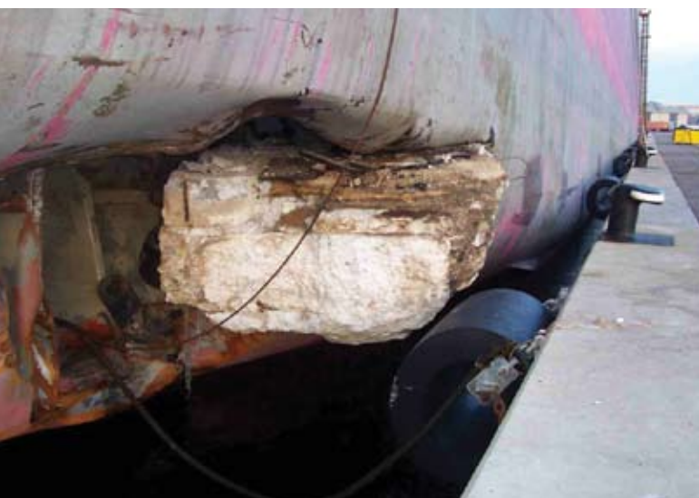
Edgeless with a massive concrete block in its hull
