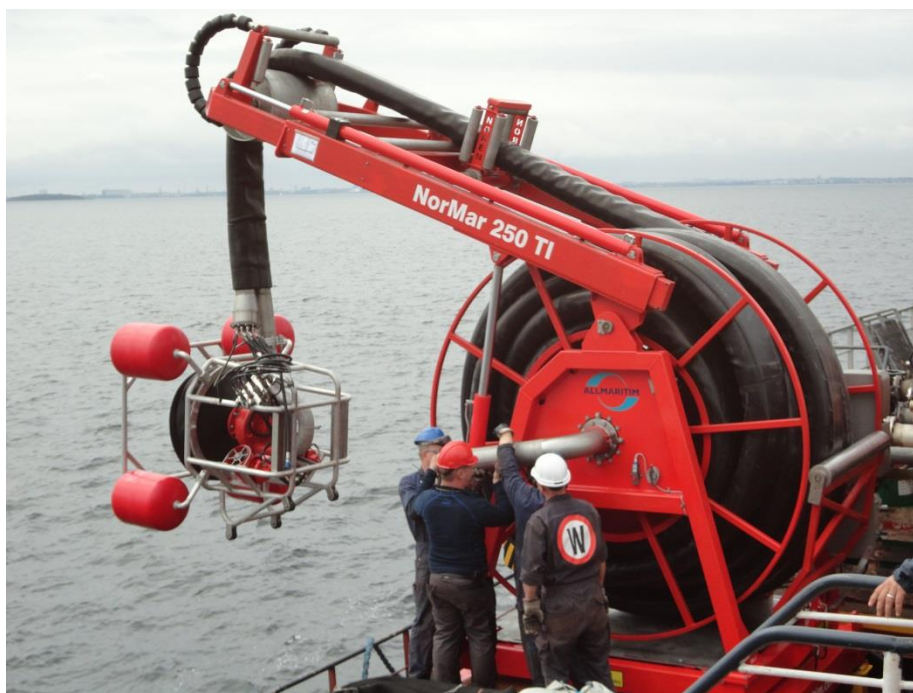
Figure 1. Quarterly drill on board OW Copenhagen - deployment of the NorMar 250 TI skimmer
