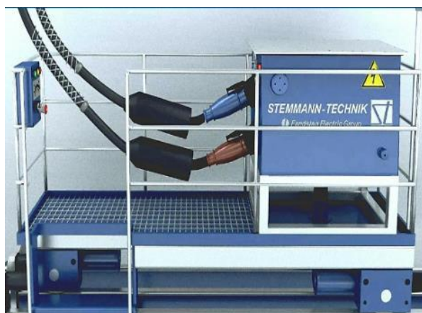
Figure 3.121 and Figure 3.122– To provide for longitudinal flexibility at berth, a mobile socket-outlet junction box can be considered in order to allow for cables to be provided by the ship-side at the most convenient location.
