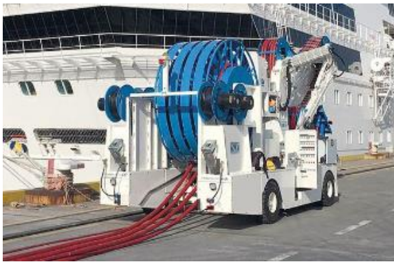
Figure 3.110 and Figure 3.111 – OPS mobile CMS – Port of Shanghai.
