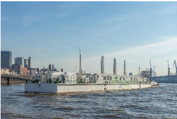
Figure 3.2 – Floating port generator.
