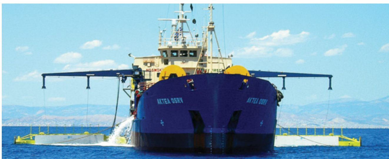
Figure 12 - Aktea OSRV, oil tanker, one of EMSA's Stand-by Oil Spill Response Vessels
