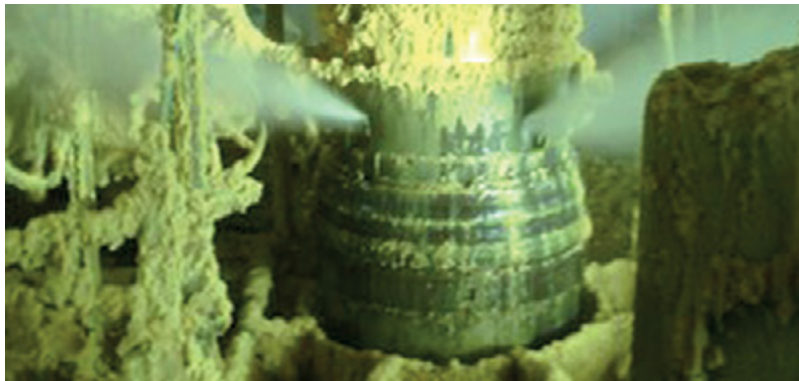
Figure 5 - Photo taken by the Wild Well Control/Total reconnaissance team reveals four leaks releasing 200,000 cubic metres of natural gas a day. 63
