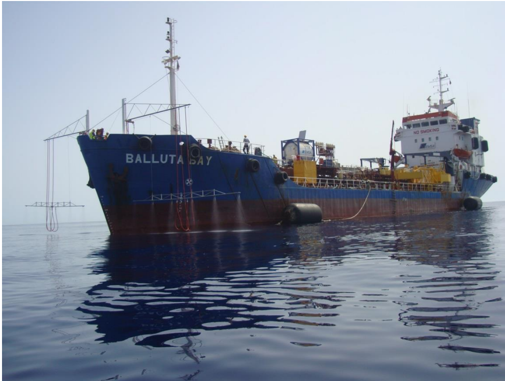
Figure 4 Dispersant spraying system deployed from the Balluta Bay during sea trials
