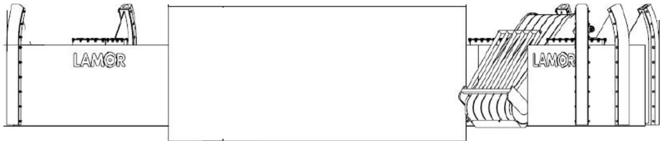
The construction is made of aluminium and steel. The oil guiding plate is of polyethylene, an easy to clean, glossy surface where the oil does not stick.
