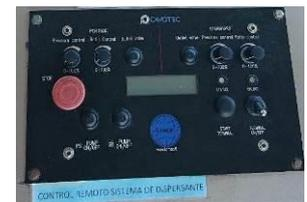
**3.4.4 Remote control - Remote Cable Control System, EX Zone I for Dispersant Spray Pump**
