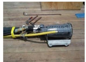
Hydraulic control valve with TEMA connectors, GTA 115
