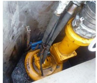
The Marflex pump type MSP-150 is a hydraulically driven portable single stage vertical centrifugal pump that has been designed for efficient handling of viscous liquids, bulky solids and shear-sensitive liquids. The MSP 150 portable pump is based upon a centrifugal screw impeller that combines the properties of a screw pump with those of a centrifugal one.
