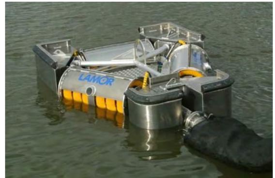
The skimmer is manufactured from aluminum with 3 specially designed hollow floats with internal chambers.
