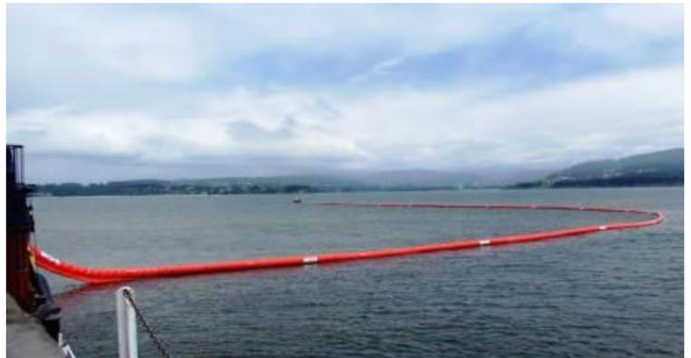
The Ocean Master 1900 is an automatic oil boom designed for open waters and offshore applications. The boom is designed for significant wave heights up to 3.5 m and wind speeds up to 25 m/s.
