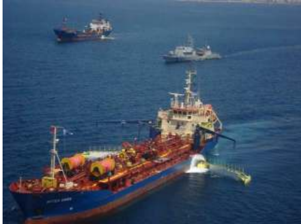
M/T Mistra Bay , the Coastguard boat and M/T Aktea OSRV with the sweeping arms deployed
