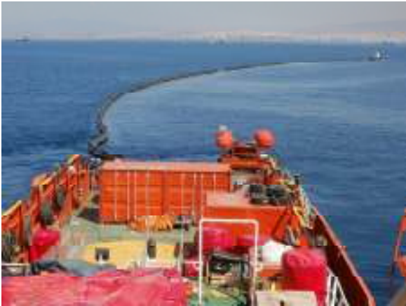
500 m boom deployed from the M/V Aegis
