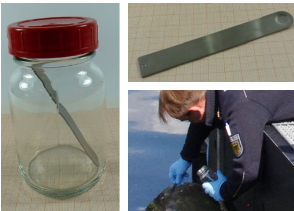
Figure 9: Stainless steel spatula and its use for scrape sampling. Credits: U. Kraus, BSH
