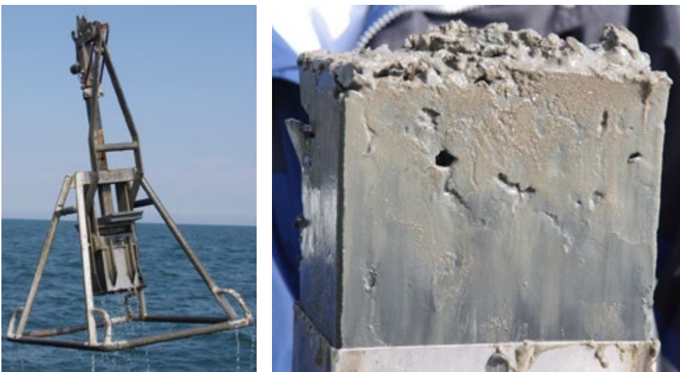
Figure 18: A box corer used for taking samples from the sea floor (left) and a sediment core extracted from the sea floor (right). Credits: U. Kraus, BSH
