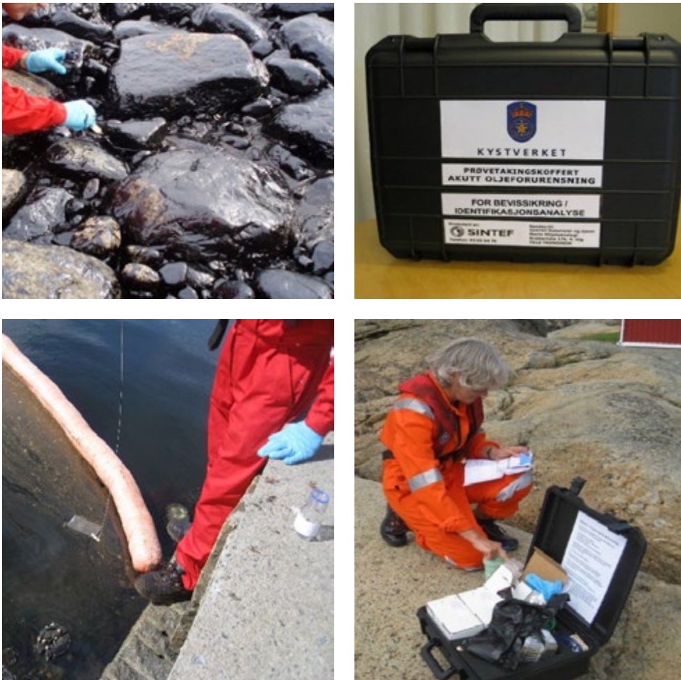
Figure 25: Pictures of sampling and sampling equipment used for securing of evidence for oil identification. Credits: Norwegian Coastal Administration
