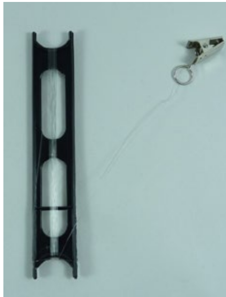
Figure 6: Nylon line with stainless steel clip (single use article). Credits: U. Kraus, BSH
