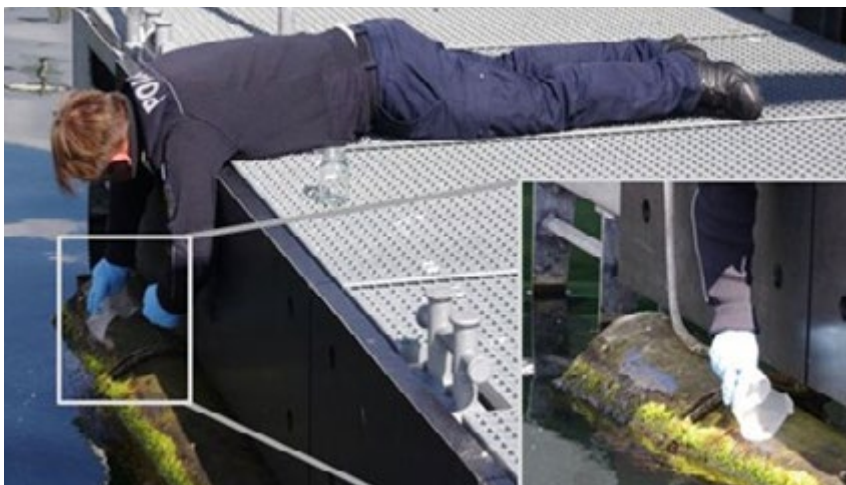
Figure 8: Taking a swipe sample with the ETFE net. Credits: U. Kraus, BSH
