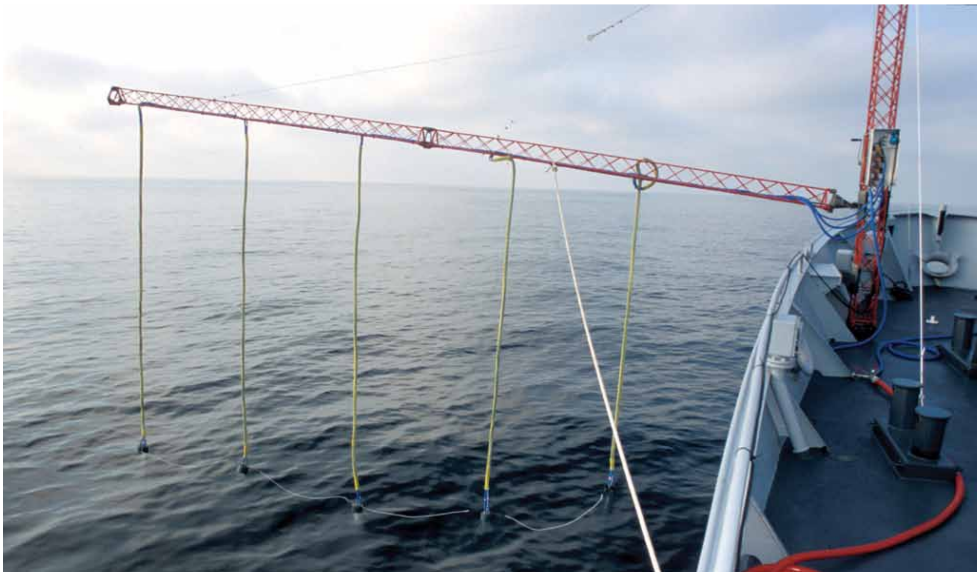
Shipboard dispersant spraying system (© Cedre).
