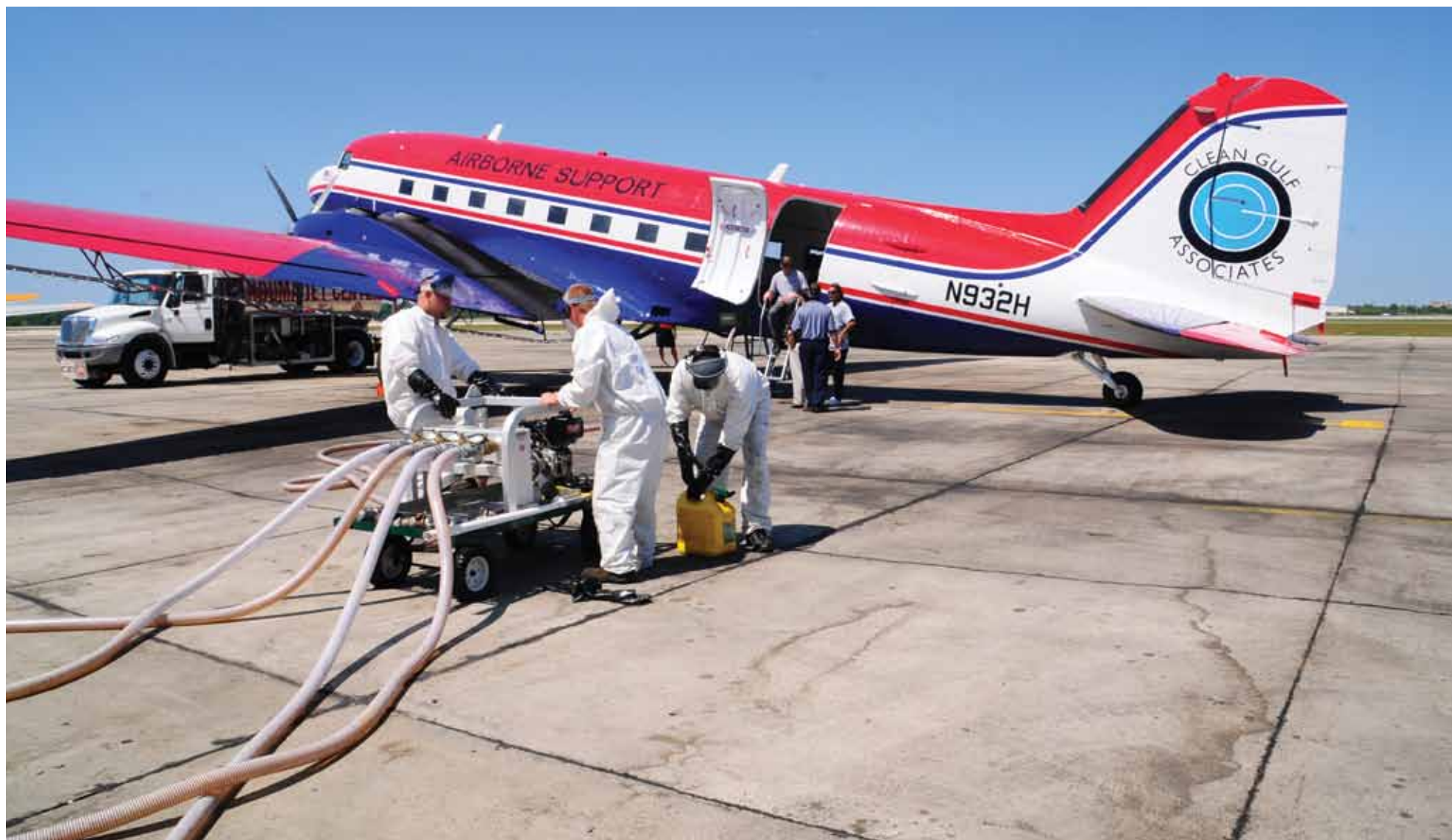
Oil dispersant is carefully pumped from tanks into a Basler BT-67 fixed wing aircraft, which will deploy its load over the oil spill of the Deepwater Horizon, Gulf of Mexico, May 5 2010 (© USCG by Petty Officer 3 rd class Stephen Lehmann).
