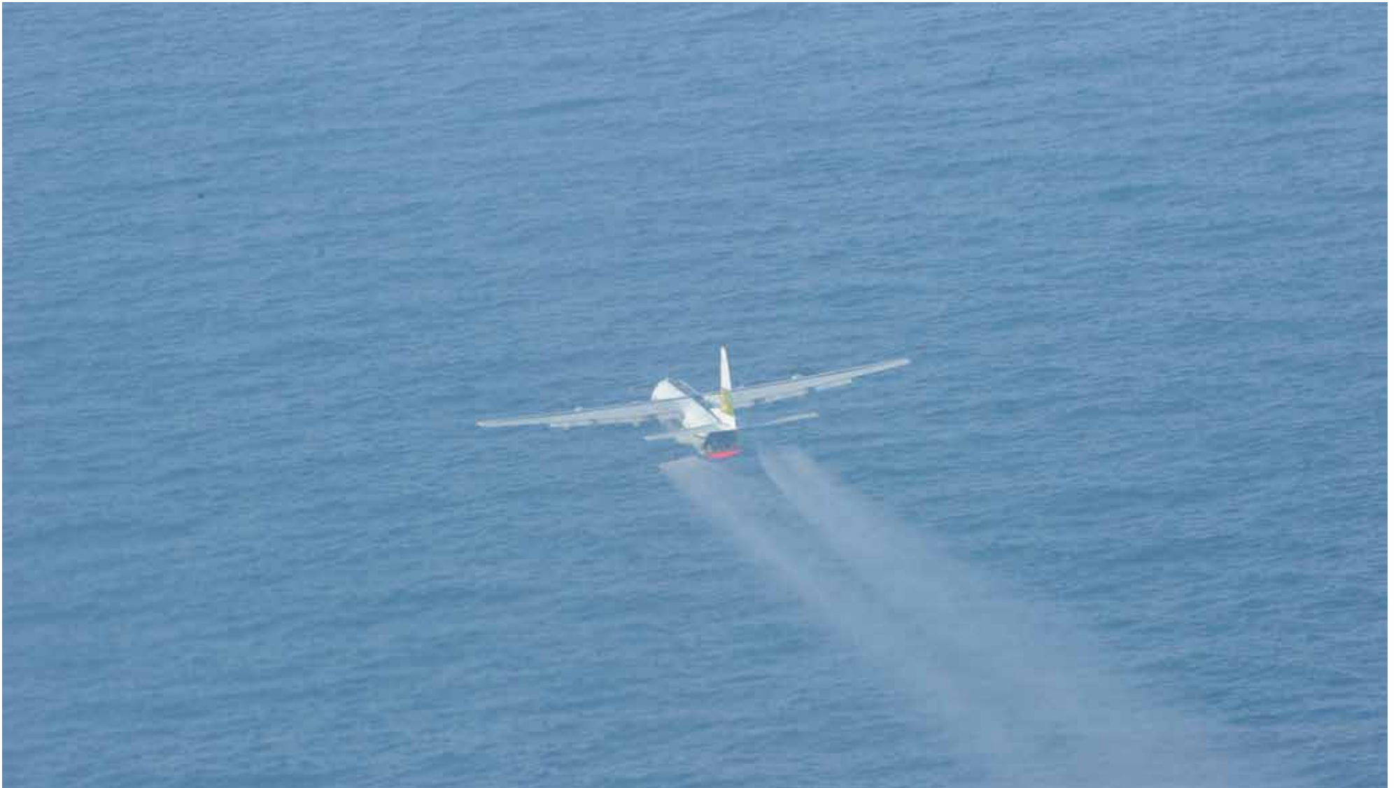
Marine Spill Response Corporation's C-130 aircraft sprays dispersant on an oil slick south of the Mississippi coastline. The U.S. Coast Guard is working in partnership with BP PLC, local residents and other federal agencies to aid in preventing the spread of oil following the April 20 explosion on mobile offshore drilling unit Deepwater Horizon. (© USCG by US Navy Mass Communication Specialist 2nd Class (AW/SW) Jonathen E. Davis).
