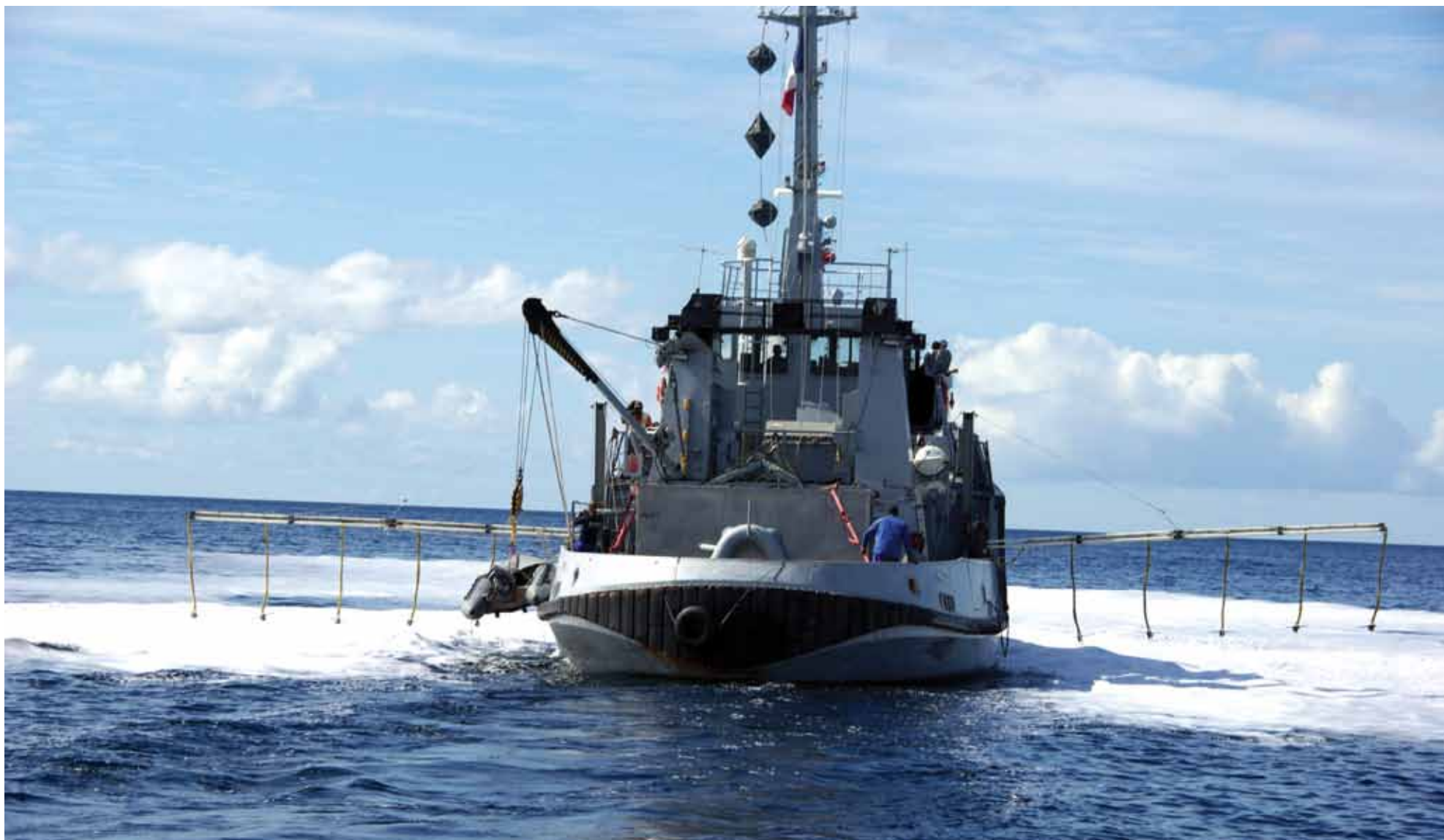
Shipboard dispersant spraying system, during an exercise near Saint Barthélemy, French West Indies (© Cedre).
