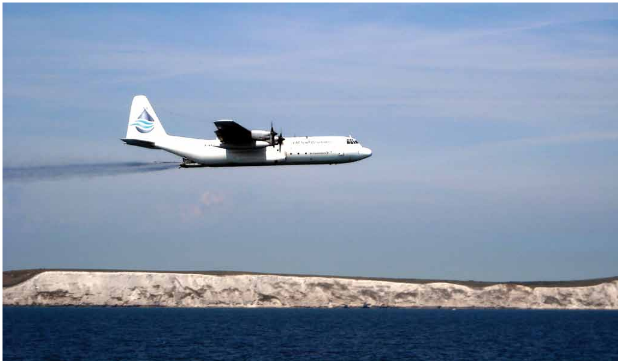
Aerial dispersant spraying during an exercise near the Isle of Wight, United Kingdom with the OSR Hercules which is equipped with an ADDS pack system (© Cedre).
