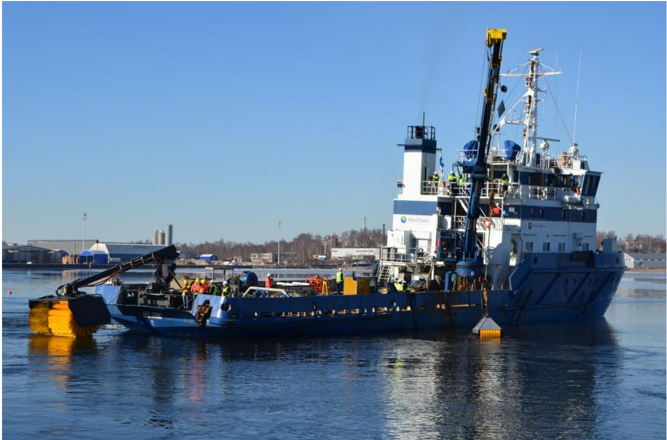
Figure 1. Seili with the SYKE ice skimmer (stern) and the Lamor LAS 125 Arctic Skimmer deployed.
