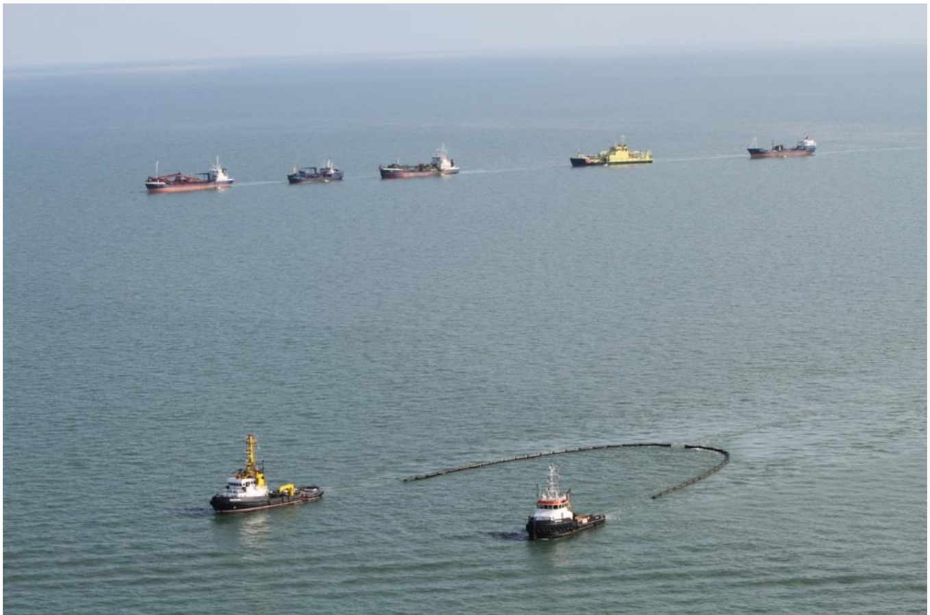
Figure 9. Tugs Zeehound and Zetiger towing boom in "U" formation. Vessels in column (from the left): DC Vlaanderen 3000 , Interballast III , Rio , Arca and Interballast I
