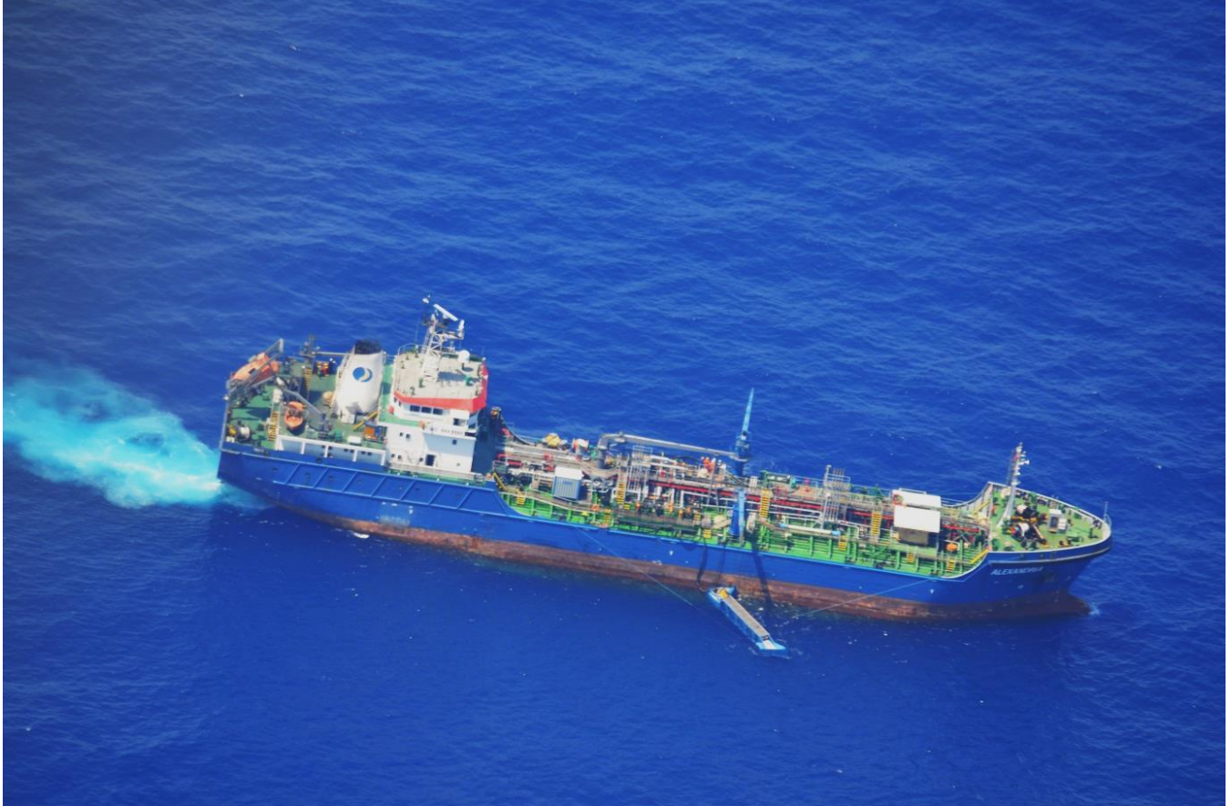
Figure 2. Alexandria performing oil recovery with the sweeping arm system.
