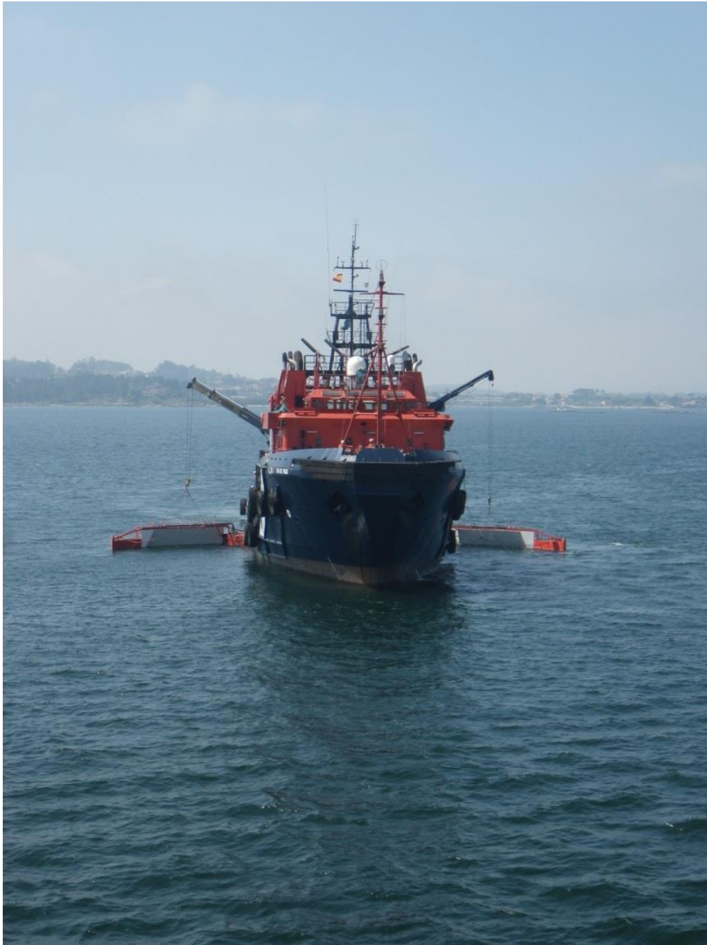
Figure 4. Ría de Vigo with the sweeping arms deployed
