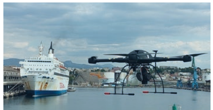
EMSA sniffer drone supporting French authorities to monitor ship emissions on Mediterranean Sea coast.
