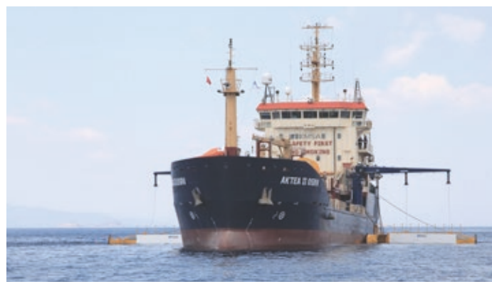
View of the Aktea II OSRV with both sweeping arms deployed
