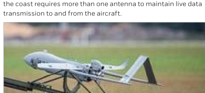
No runway is needed for this particular fixed wing RPAS which is launched from a catapult and recovered with a net
