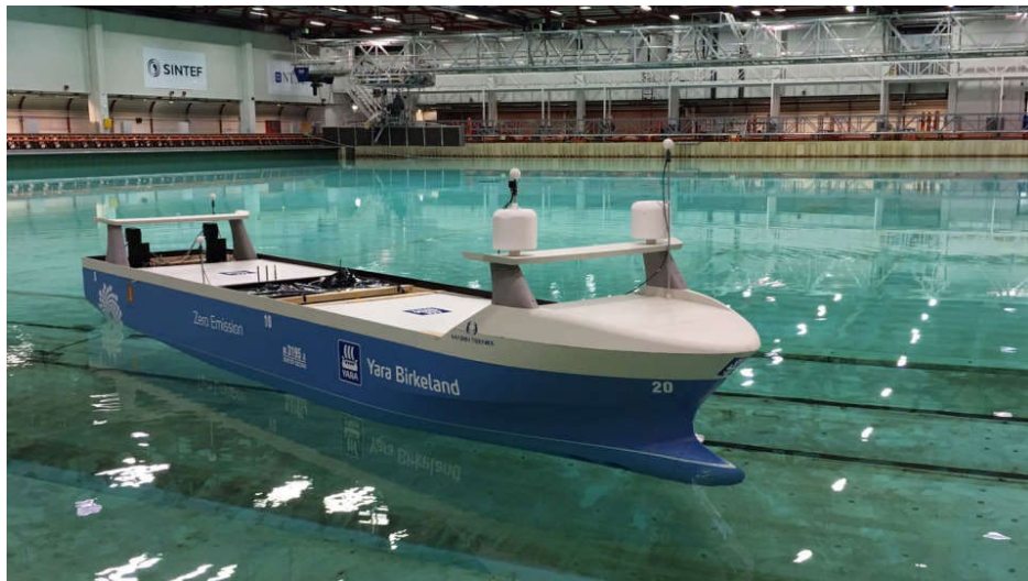
Figure 2-15 Model of the final design of the autonomous and fully electric container vessel, Yara Birkeland, in the test tank facility at SINTEF Ocean (Kongsberg Maritime, 2017)
