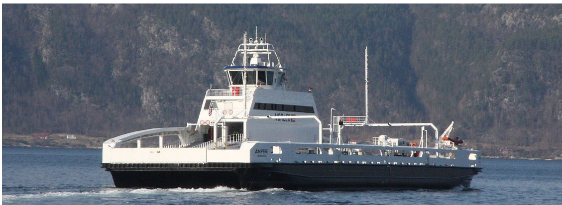
Figure 2-5 The world's first large-size all-electric battery-powered car ferry, MF Ampere
