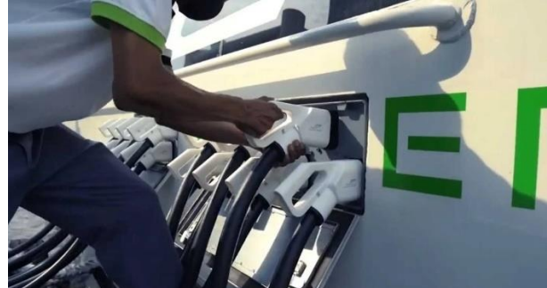
Figure 8.9 (a) and (b) – MINE Smart Ferry – Thailand- use of 26 CCS type charger connectors for fast charging of a passenger ferry.
