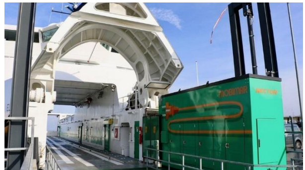
Figure 8.11 – AERO MV Ellen – Fast DC charging by the bow. Different connection solution.
