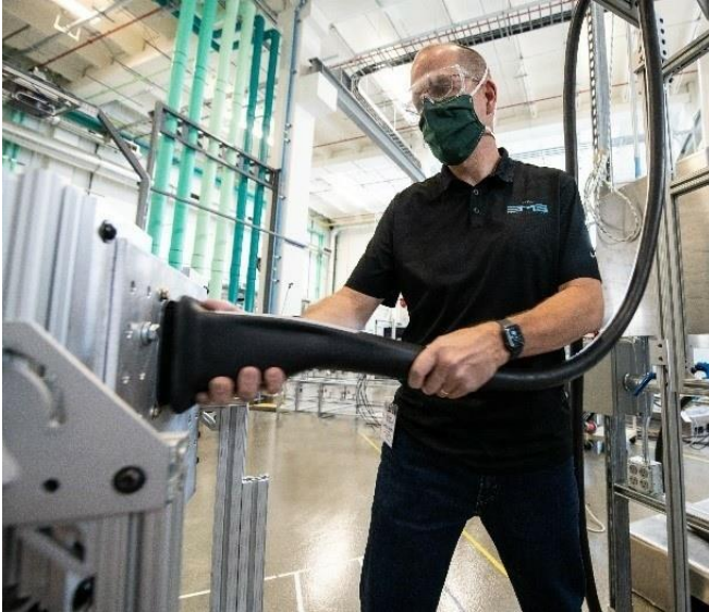
Figure 5.5– Multi-MW Charging System (MCS) under development and under tests in laboratory. Designed to meet the needs of heavy-duty trucks.
