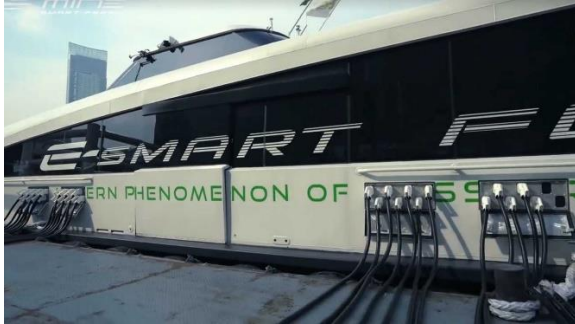
Figure 8.9 (a) and (b) – MINE Smart Ferry – Thailand- use of 26 CCS type charger connectors for fast charging of a passenger ferry.
