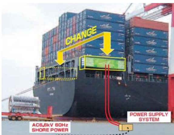
Figure 4.9 – HV Shore Power solution from containership.
