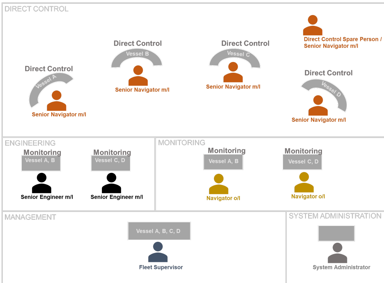
Figure 28: Example ROC Design for "Ferry on short passages".
