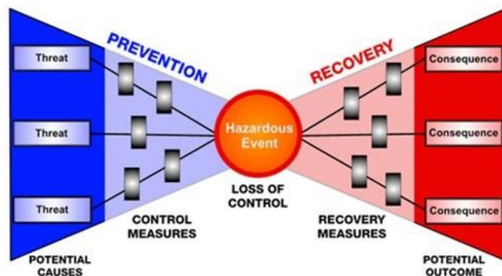
Figure 2.5-1. Illustration of the Bow Tie model, a barrier risk model for identification and management of hazards.
