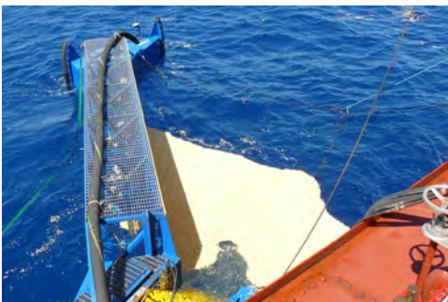
The GALP Marine simulating the collection of oil (pop corn) with the port sweeping arm during the exercise
