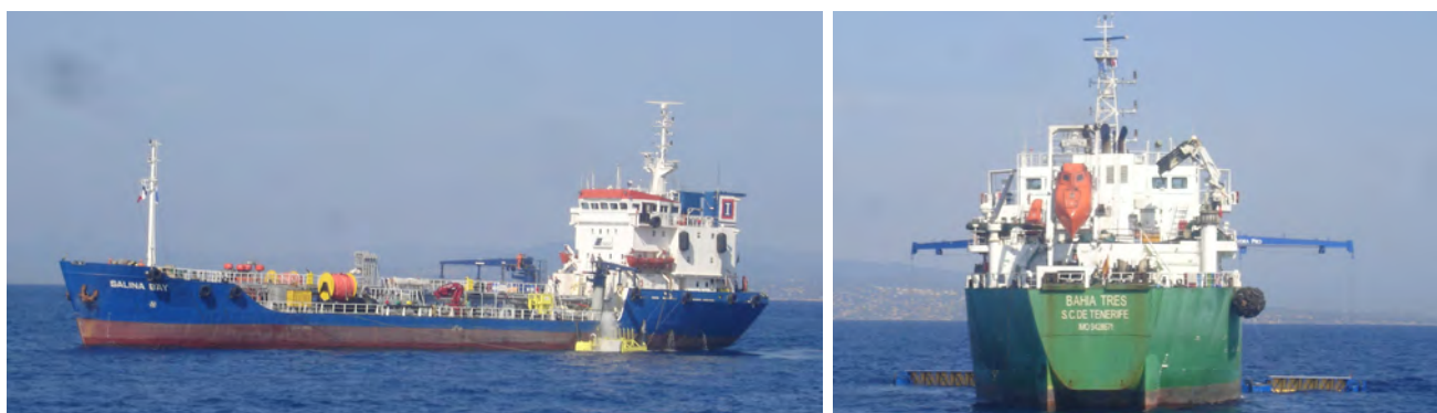
Salina Bay (left) and Bahia Tres simulating oil recovery with sweeping arms deployed
