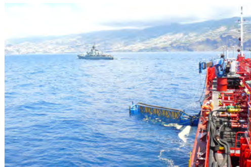
The GALP Marine simulating the collection of oil (pop corn) with the port sweeping arm during the exercise
