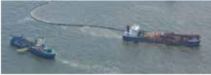
The hopper dredgers, Interballast III (storage capacity 1,886 m 3 ) and DC Vlaanderen 3000 (storage capacity 2,744 m 3 ), operate along the Belgian and Dutch coastlines.
