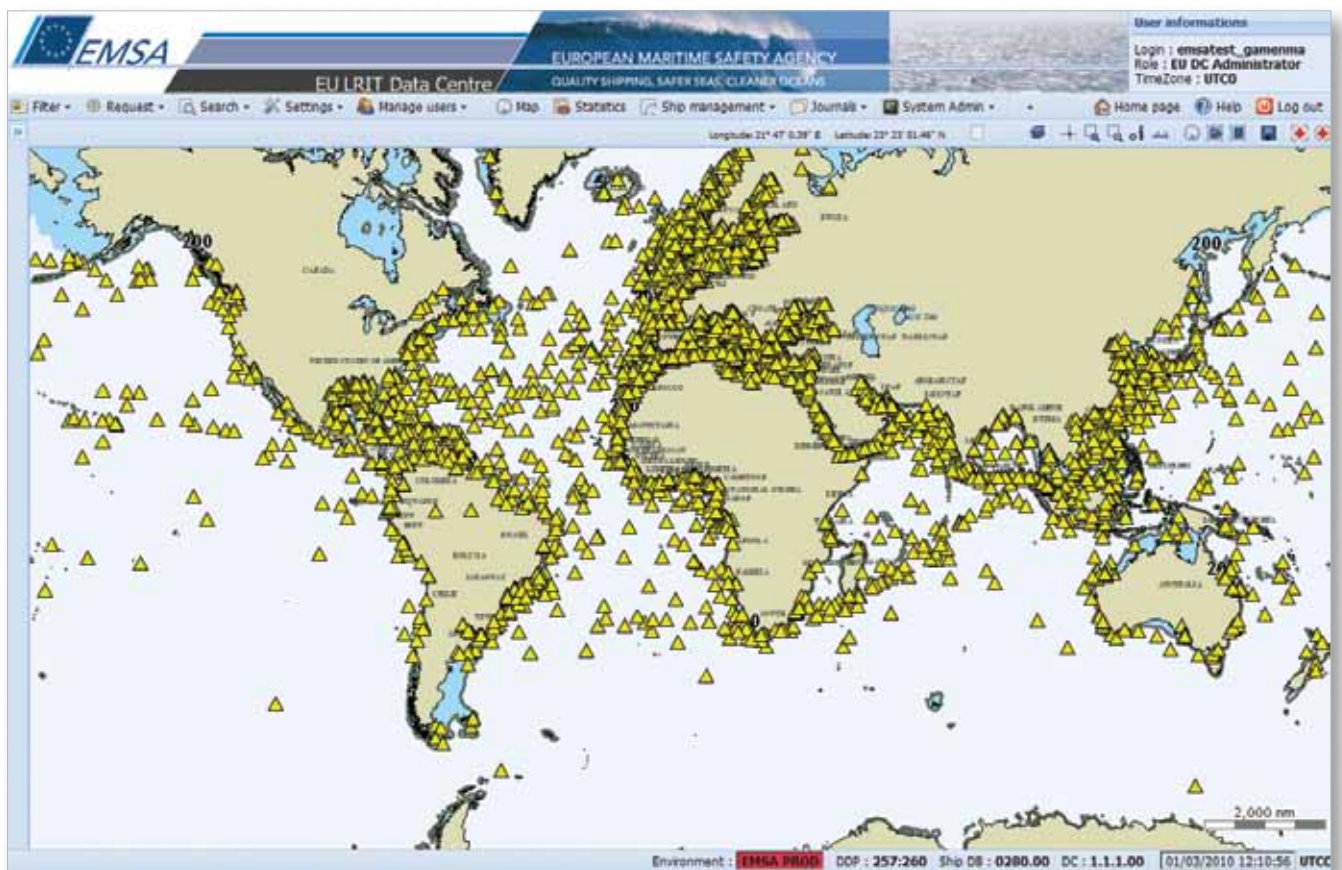
Each yellow triangle on the LRIT interface represents a ship flying the flag of a participating country (EU LRIT CDC).
