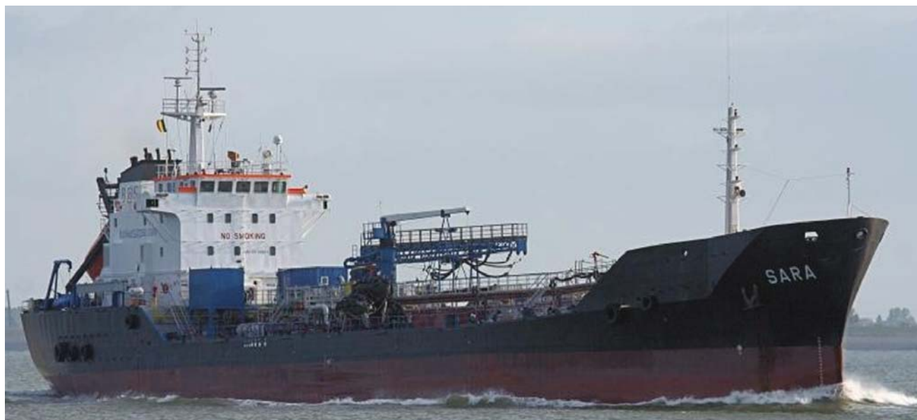
Double-hulled bunker tanker Sara was contracted at the end of 2009. She will be prefitted in 2010 to provide at-sea oil recovery services (capacity for recovered oil of 6,658 m 3 ) for the Atlantic front.
