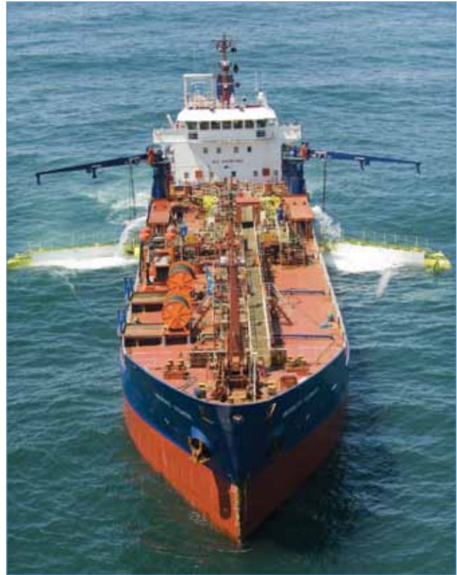
The Mersey Fisher deploys sweeping arms during an exercise. This oil spill response vessel is on stand-by for the Atlantic Coast.
