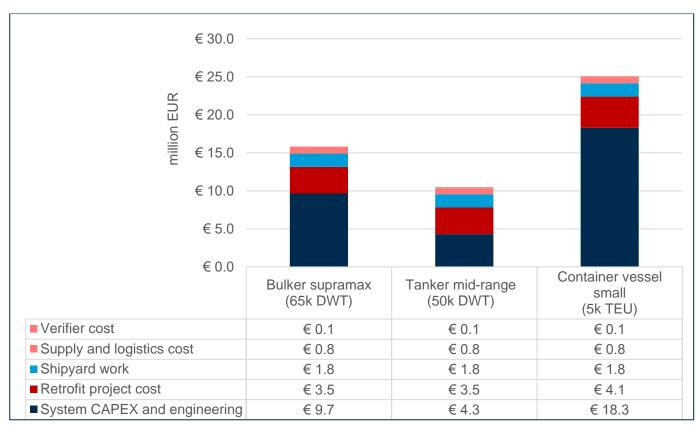
Figure 18. Total cost of retrofitting (million EUR) conventional fuel to hydrogen ICE system
