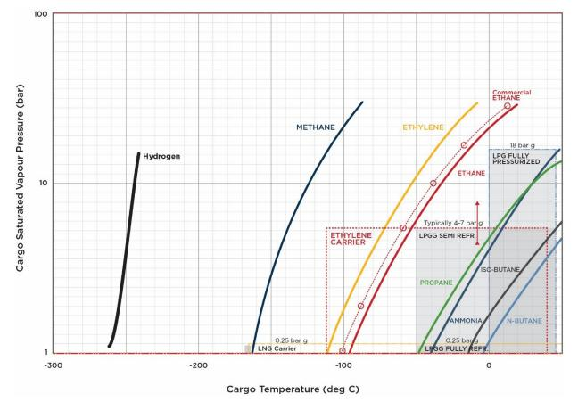
Figure 22. Typical operating range for Liquefied Gas Carriers
