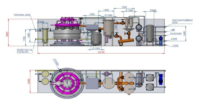
Figure 32. System General Arrangement
