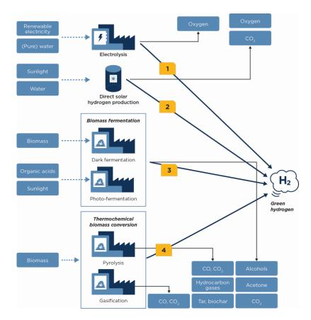
Figure 1. Production pathways for green hydrogen.
