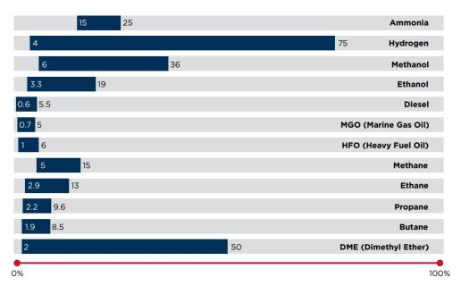
Figure 10. The flammability ranges for different fuels in % volume with air (ABS, Sustainability Whitepaper, Hydrogen as Marine Fuel, 2021)
