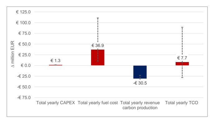
Figure 21. Additional annual costs/benefits if a NG to H<sub>2</sub> decomposer system is installed and used on an LNG carrier
