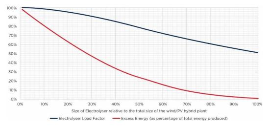
Figure 4. The relationship between the electrolyser's load factor and excess renewable electricity, given the sizes of the system and wind/solar park (IEA, 2017)
