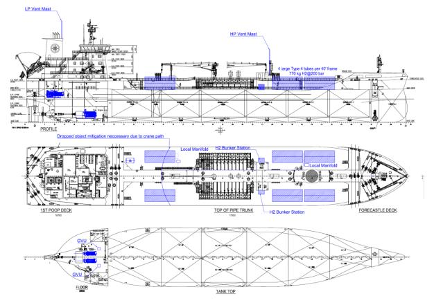
The fuel piping from each fuel storage tank on the weather deck runs alongside the pipe trunk.
