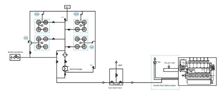
Figure 8. Schematic integration of the FSS for a 4-stroke Otto-cycle hydrogen engine
