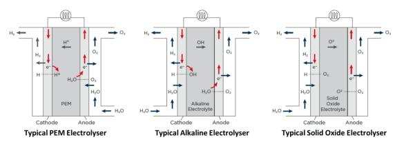
Figure 2. Electrolyser technologies currently available or under development (ABS, SETTING THE COURSE TO LOW CARBON SHIPPING)
